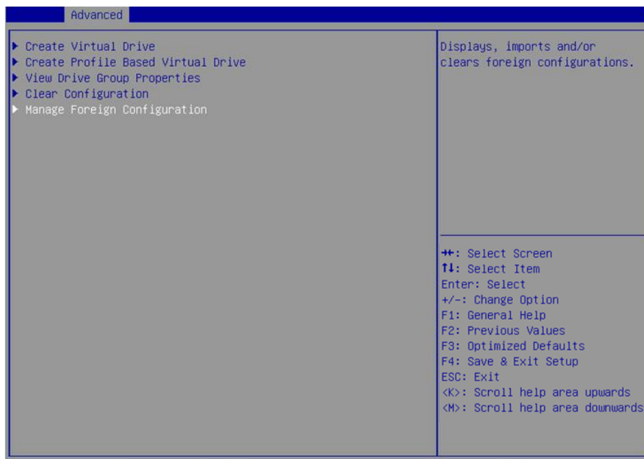
図93 Foreign Configurationの選択
